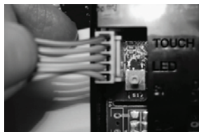
Figure 27 - Connecting end of Touch Pad Cable
