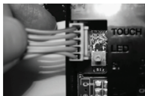
Figure 20 - Connecting end of Touch Pad Cable
