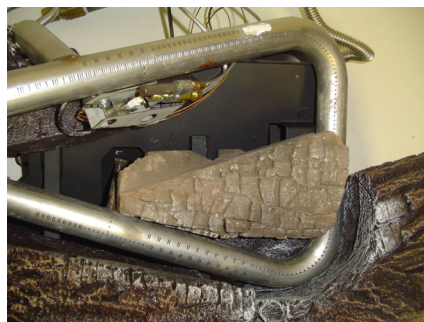
Figure 27A - Installing Charred Log Top View
