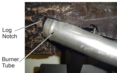
Figure 25A - Installing Back Left Log
