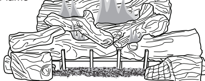
Figure 71 - Incorrect Front Burner Flame Pattern
