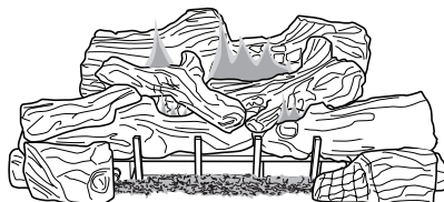
Figure 70 - Correct Front Burner Flame Pattern
