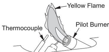
Figure 27 - Incorrect Pilot Flame Pattern
