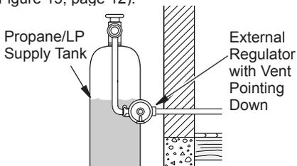
**Figure 14 - Equipment Regulator with Vent Pointing Down**
