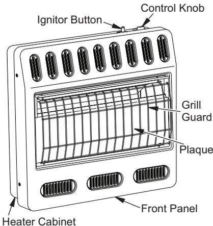
**Figure 1 - Vent-Free Gas Heater**
