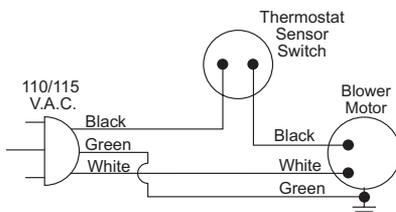
Figure 25 - Wiring Diagram for Blower Accessory
