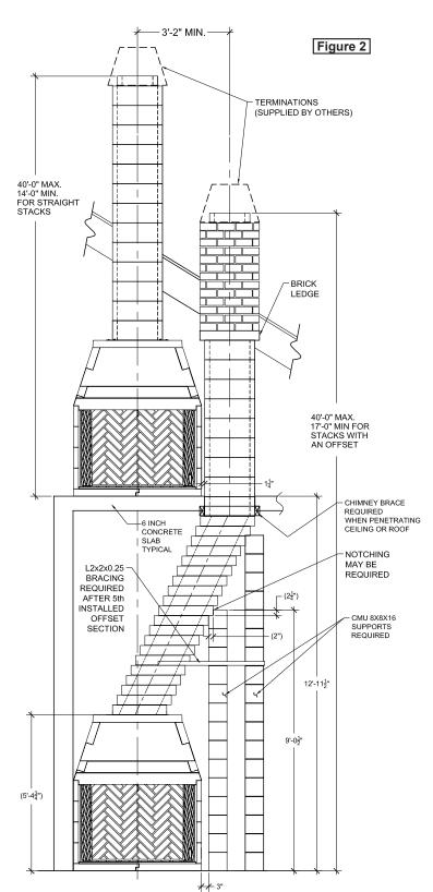
The Masonry Chimney System consists of the following components:
