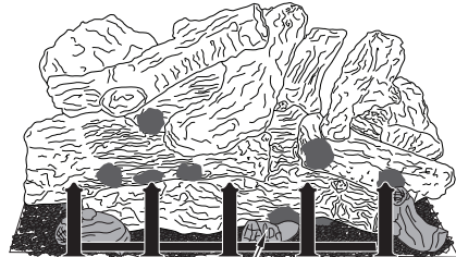
Figure 31 - Installing Scrap Log Pieces
