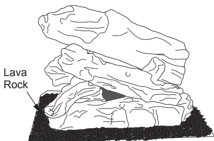
Figure 29 - Installing Lava Rock
