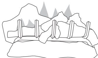
Figure 18 - Correct Burner Flame Pattern
