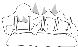
Figure 45 - Correct Burner Flame Pattern
