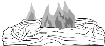
Figure 36 - Incorrect Burner Flame Pattern
