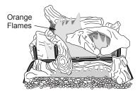
Figure 24 - Incorrect Burner Flame Pattern
