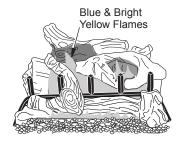
Figure 23 - Correct Burner Flame Pattern
