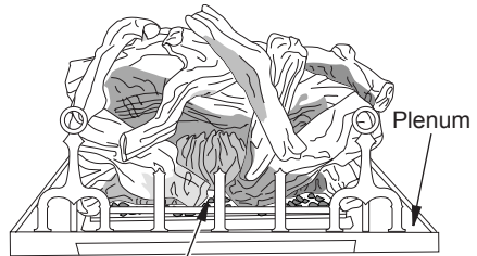
Ember Material Figure 38 - Placing Ember Material on Burner
