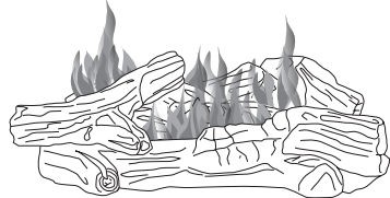
Figure 34 - Incorrect Flame Pattern with Control Knob Set to High Flame
