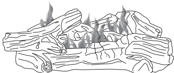
Figure 38 - Correct Flame Pattern with Control Knob Set to High Flame.
