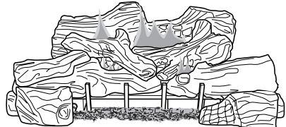
Figure 39 - Correct Front Burner Flame Pattern
