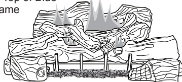
Figure 41 - Incorrect Front Burner Flame Pattern
