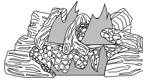
Figure 51 - Typical Flame Pattern
