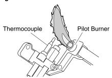
Figure 19 - Incorrect Pilot Flame Pattern
