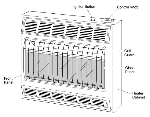
Figure 1 - Vent-Free Natural Gas Heater (Models VN2800BTD Shown)
