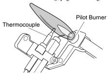
Figure 18 - Correct Pilot Flame Pattern
