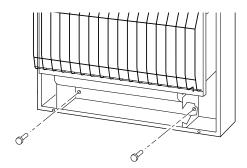
Figure 12 - Installing Bottom Mounting Screws
