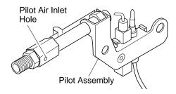
Figure 22 - Pilot Inlet Air Hole
