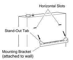
Figure 11 - Mounting Heater Onto Mounting Bracket
