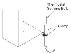
Figure 5 - Attaching Thermostat Sensing Rulb
