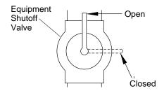
Figure 14 - Equipment Shutoff Valve
