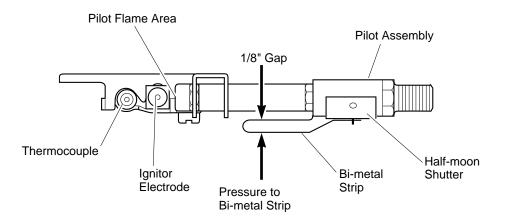
This adjustment process must be completed after maintenance or cleaning has been performed to insure proper setting of the cold choke.
